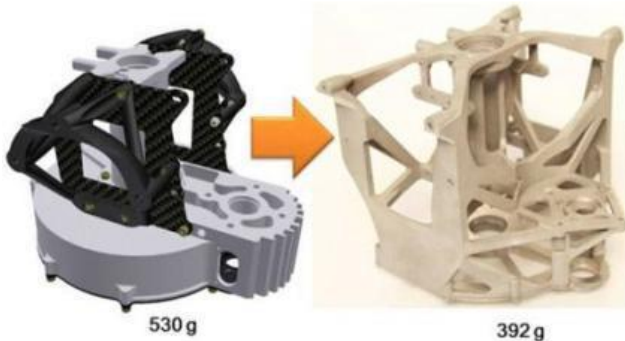
Flying Cam part - SIRRIS redesign – MBProto LBM building (Compolight)
