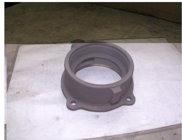
Magnesium Seal housing of Kaveri engine (GTRE, Bangalore) made by Aerocast, France
